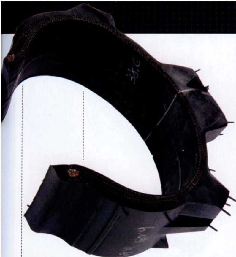
A cut-above. Cross-sections showing the metal beads and nylon plies moulded into the carcass.
